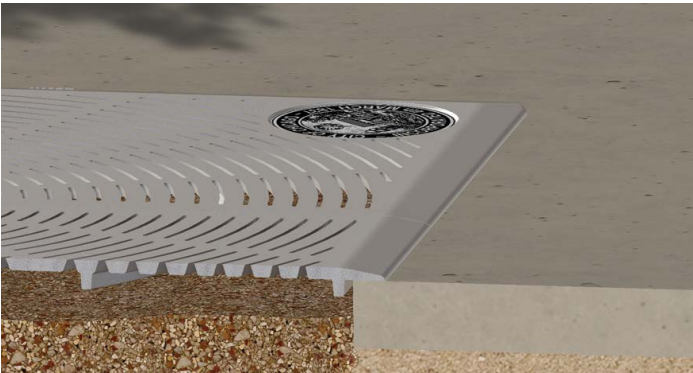
Close up section view of the retrofit tree grate. No frame required.
